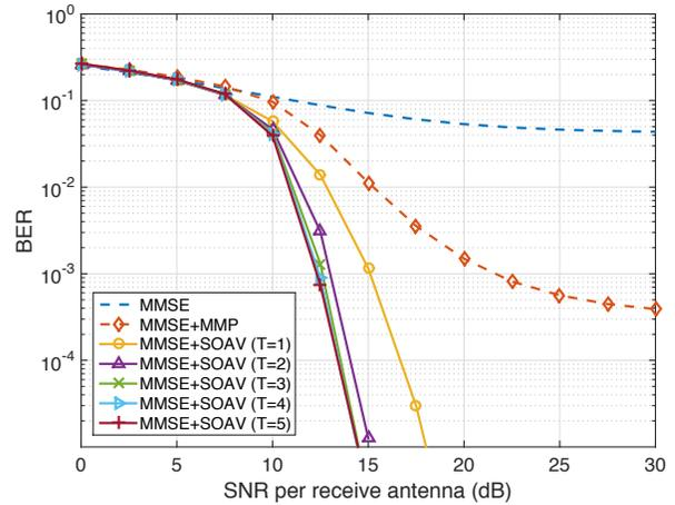
Fig. 4. BER performance for  $(n, m) = (128, 96)$
