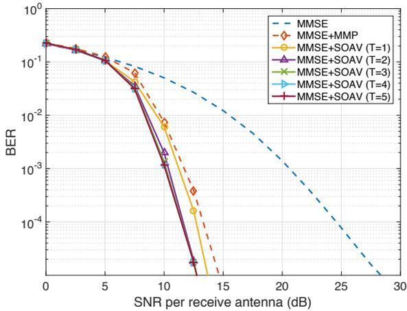
Fig. 2. BER performance for  $(n, m) = (128, 128)$
